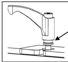
Make sure there is some space between the washer and leg when sliding it together.
