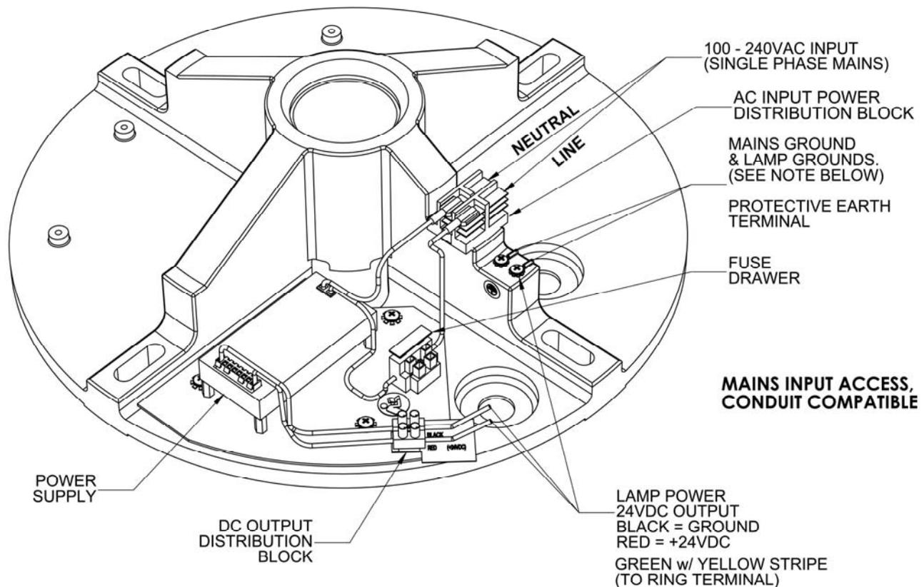
**Figure 12: Arm Cable termination**
