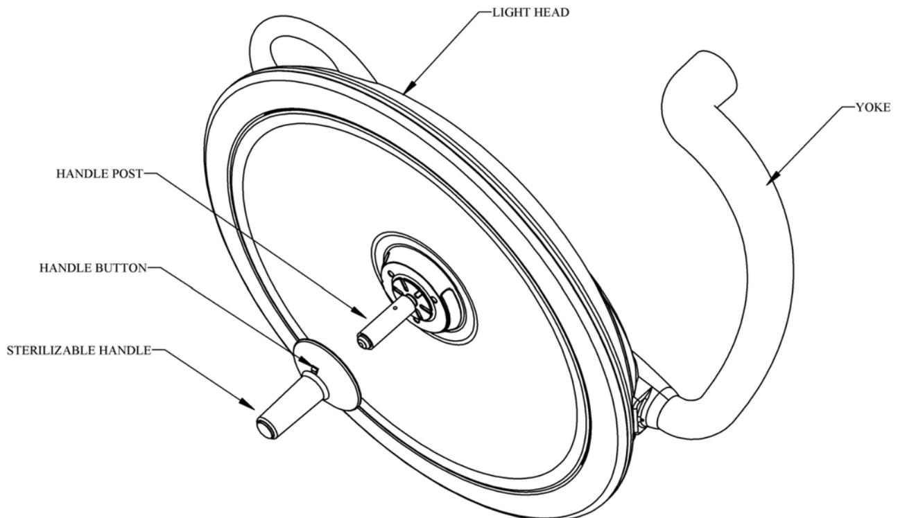
**Figure 19: Handle Sterilization**
