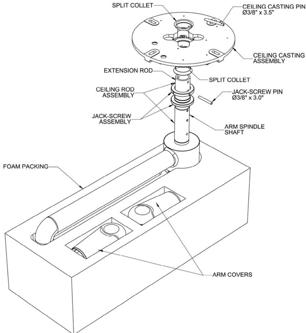
**Figure 8: Installation setup**
