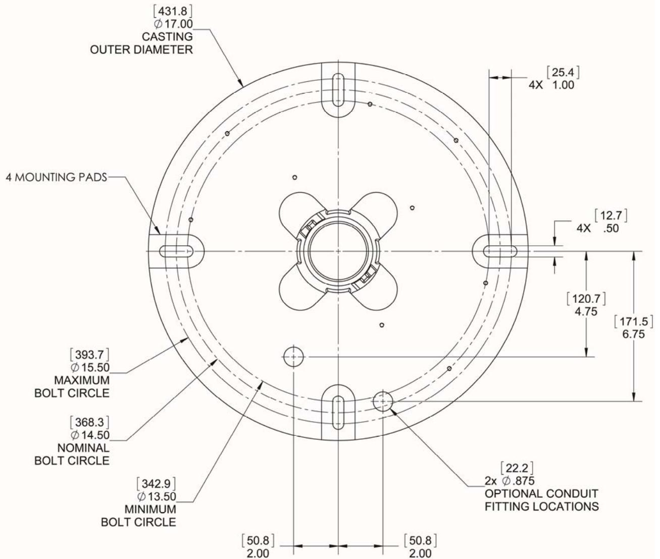
**Figure 1: Mounting Dimensions for Ceiling Casting**
