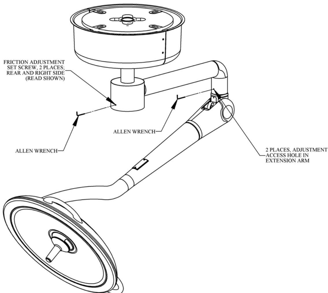
**Figure 18: Arm Friction Adjustment (solo light shown)**
