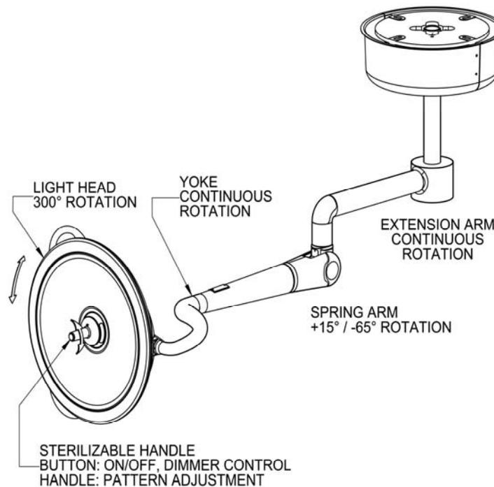
**Figure 14: Head and Arm Movement (Solo light shown)**
