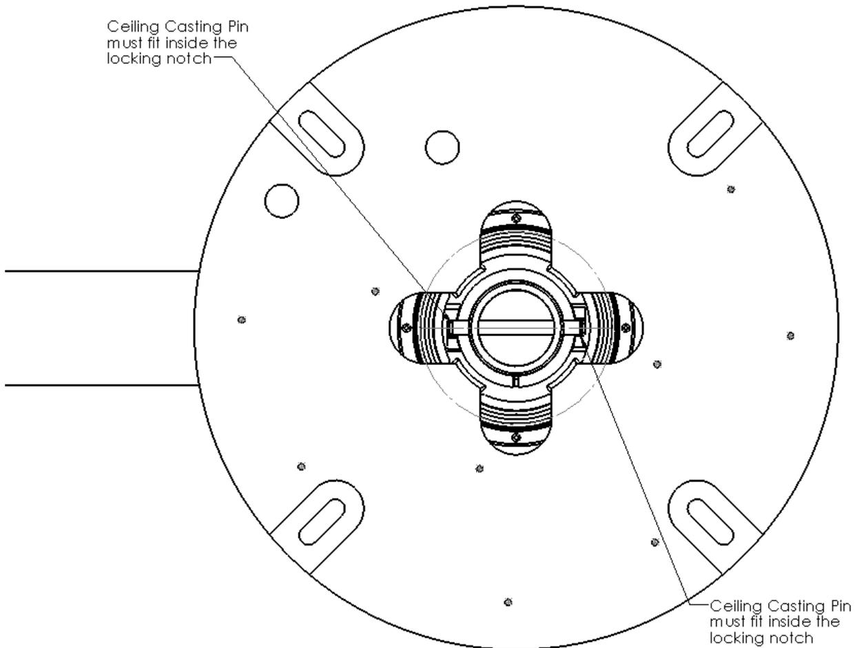
**Figure 11: Ceiling & Shaft dowel pin locking.**
