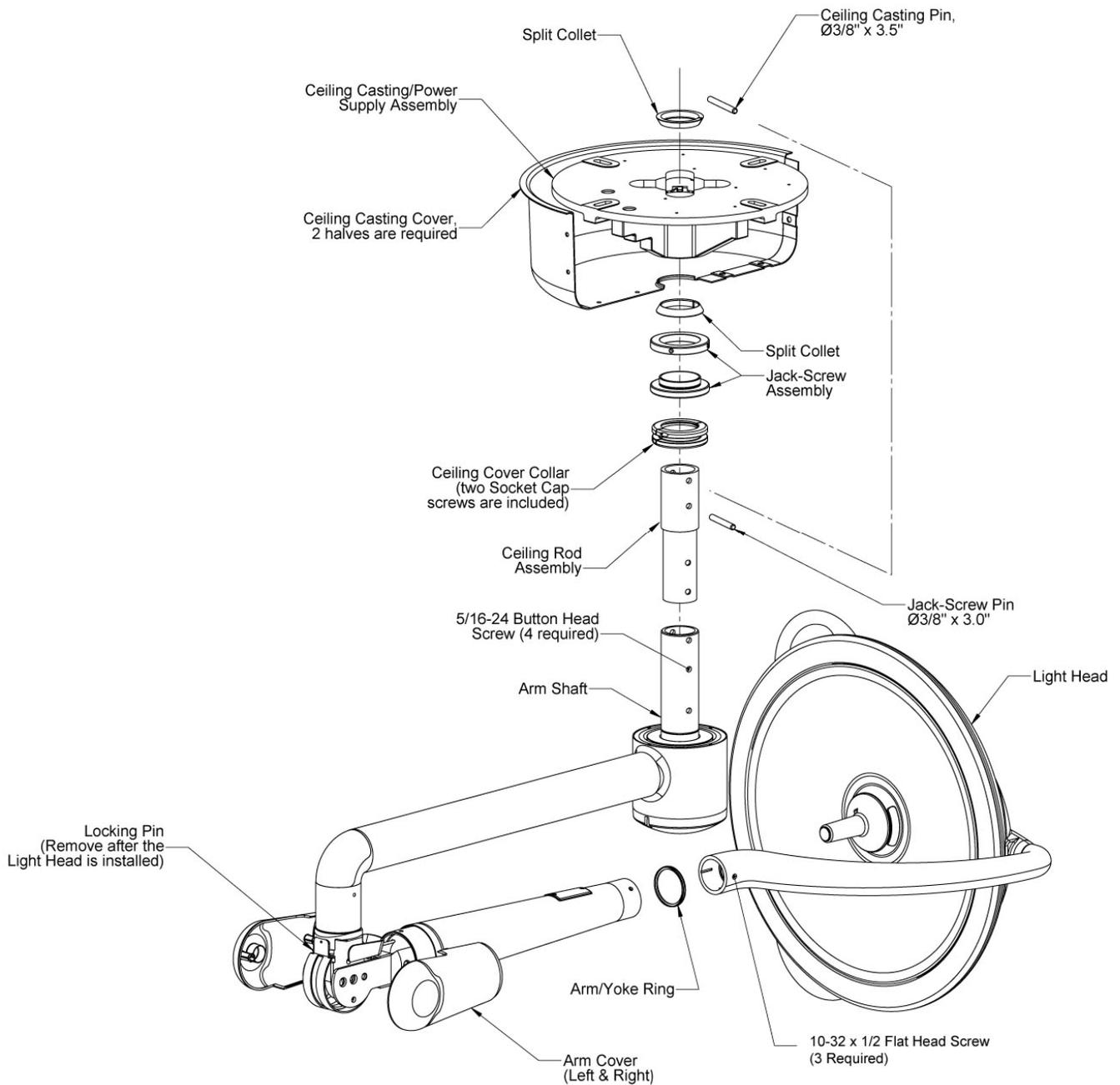
**Figure 5: Shown, sub-assemblies for a Solo, ceiling mount.**
