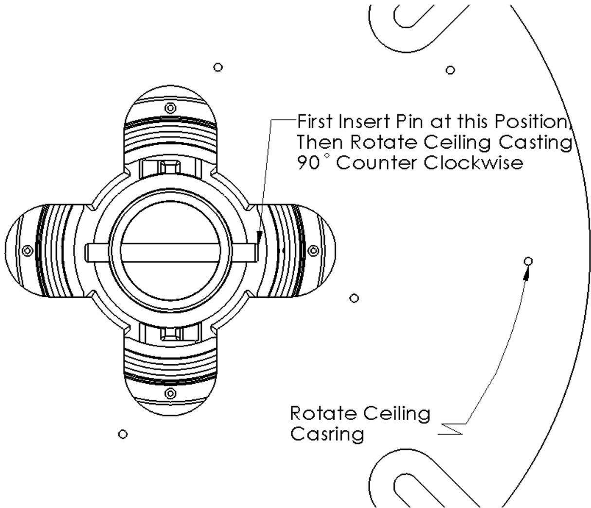
Figure 10: Ceiling & Shaft dowel pin insertion
